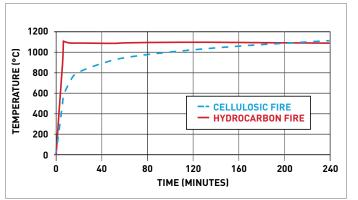
Development of a typical cellulosic fire, which consumes mostly natural materials like wood, fabrics, or paper. Material thermal response testing methods still used today rely on cellulosic fire curves substantially unchanged since 1903.
